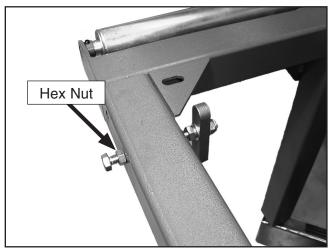
Figure 86. Crosscut fence adjustment cam.
